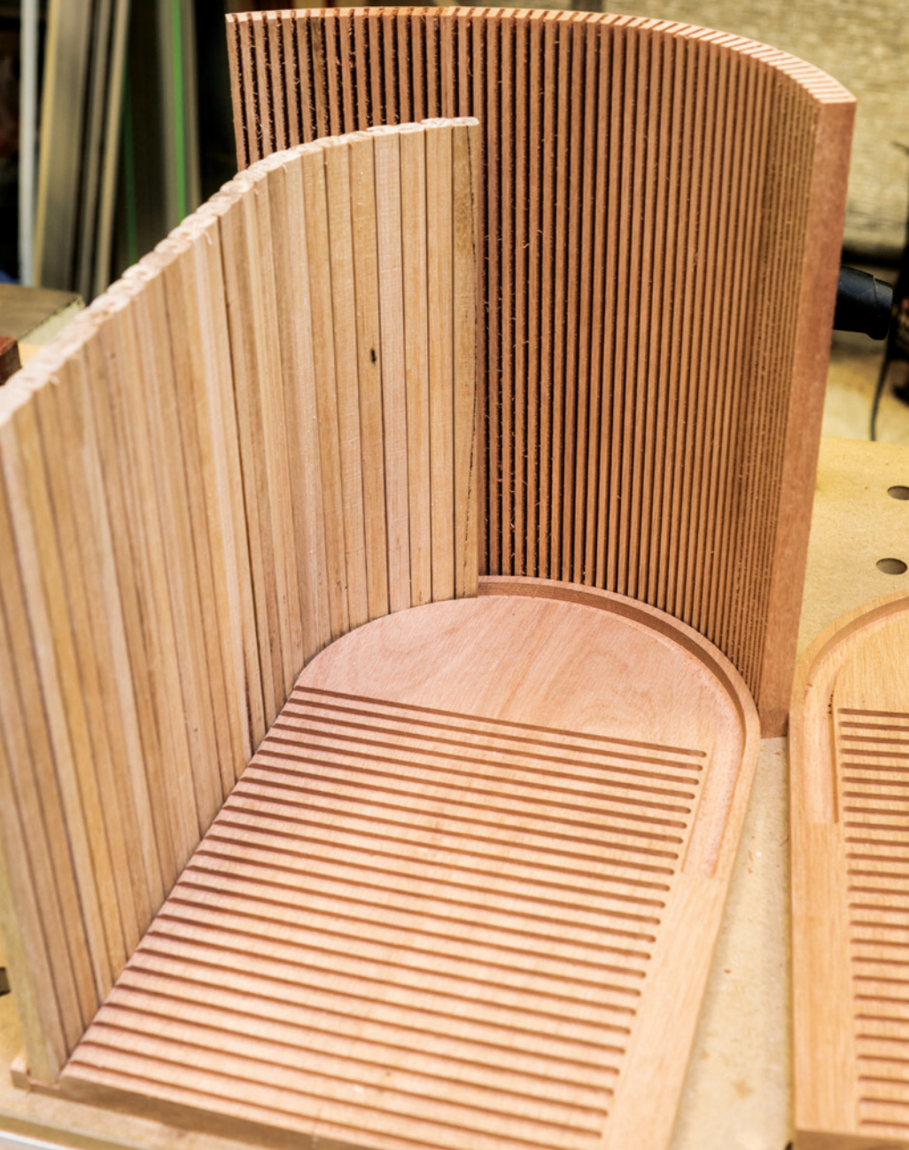
The two types of timber bending: kerfing (decorative) and tambour (mechanical).
